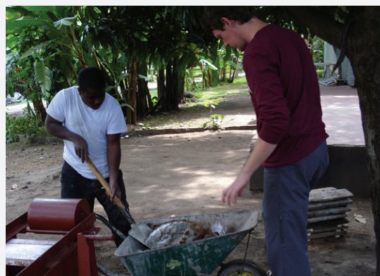
A Westlake High School student member of Engineering Without Borders mixes concrete with his GK–12 Fellow mentor for use in a brick-making machine.
